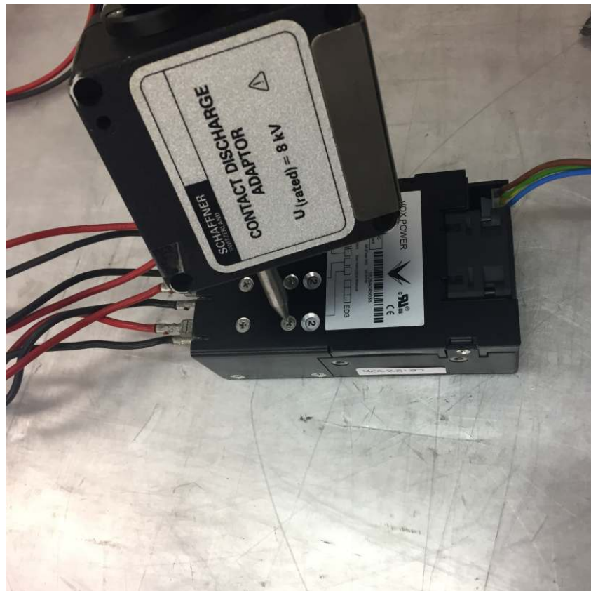
Figure 7: ESD Test Set up
